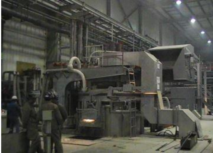
Four hole dust at the scene of the steel-making arc furnace
