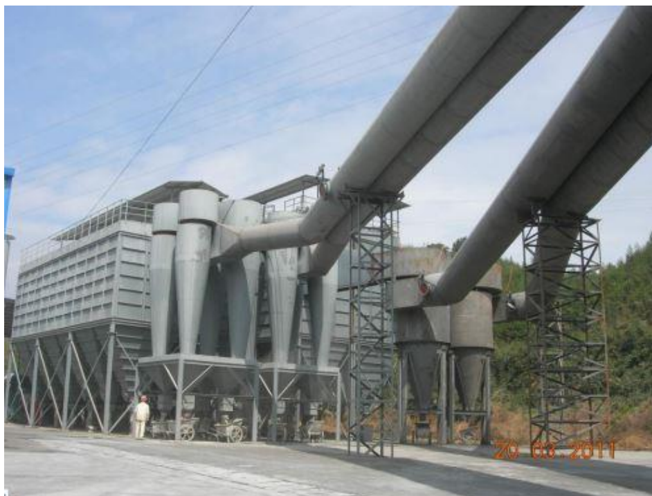
In 2009, high carbon ferrochrome dust removal equipment at the scene
